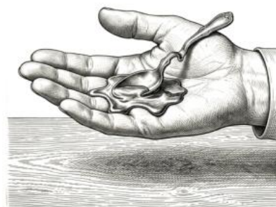
Fig. 3 — body heat crosses gallium's melting line
